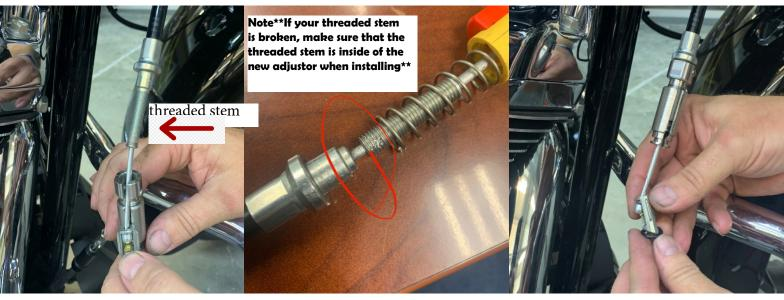
7. The new adjustor should look like the picture below when installed. After adjusting the clutch, tighten the set screw.
