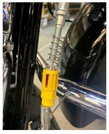
2. Remove the yellow plastic adjustor with a a pair of side cutters. Cut the plastic from the bottom and from the top. Be careful not to cut the cable wire.
