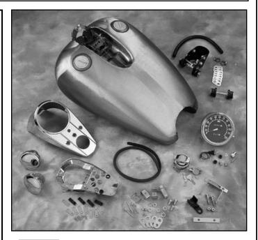
**CAUTION:** Tank should be mounted, then removed, sealed on the inside and then pressure tested before painting to prevent leaks. When mounting tank, do not stress any of the mounting tabs as this could cause failure at a later date. Use washers for shims if necessary.
