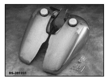
**CAUTION:** Tank should fit flush to all three mounting points. Failure to adjust the rear tank mount on the frame will allow misalignment and will place stress on the mounting tabs when mounting hardware is tightened. This can cause the tabs on the tank and frame to crack and break.
