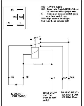
9. Turn on the ignition switch and turn to the lights position.10. Test headlight relay by pressing the momentary switch and observing if the light pattern emitted by the headlight changes. You should hear a faint "clicking" sound as the relay switches
