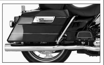
**NOTE:** There is a different muffler for the left and right side of the motorcycle. The dent in each canister should always be facing in towards the rear tire. This is to allow clearance for the swingarm and axle.
