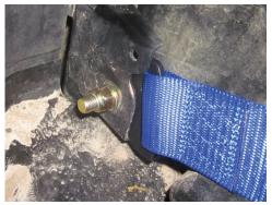
3. The upper/rear shoulder mounts will go over the horizontal roll cage tube and get bolted to the back of the harness bracket. Again, be sure to install the bolt through the bracket so it can rotate freely and torque to 25-30 ft/lbs.
