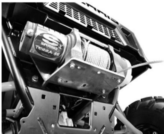
Bolt the winch in place using the hardware provided with your winch.
