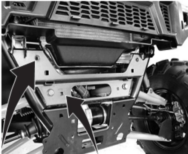
Mount will install in the top threaded holes and middle square holes with spacers in between.
