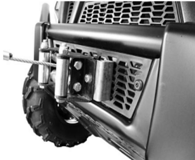
Use the roller fairlead brackets if installing a standard size fairlead or hawse.
