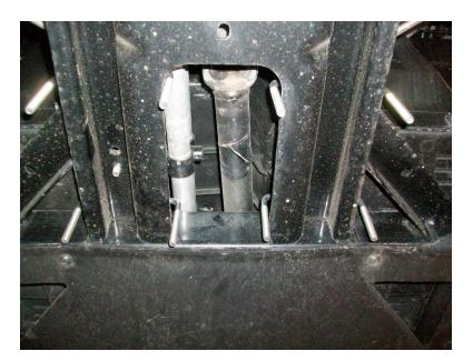
The plow mount will attach right in front of the bottom skid plate. Place the U-bolts up over the Frame as shown in picture. The rear U-bolts will go up against the frame cross member.
