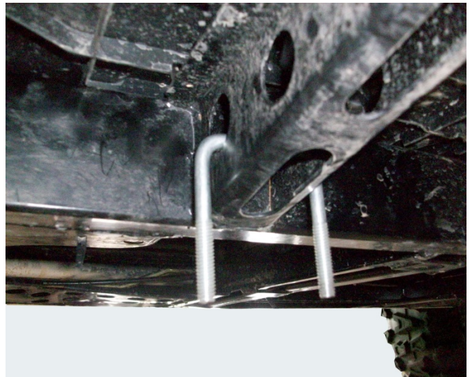
Rear U-Bolt mounting location
