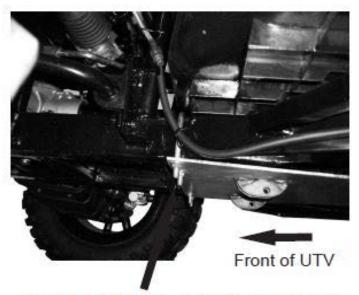
Front U-Bolt position over the main frame tubes in line with the back of the front tires
