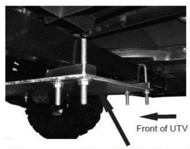
Place the spacers between the frame rail and bottom mount at the rear u-bolts.
