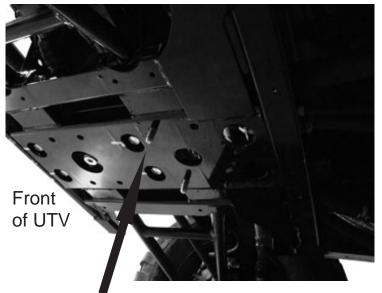
Drop the 3/8" bolts and washers down through the open holes in the frame between the steering rack and front differential.
