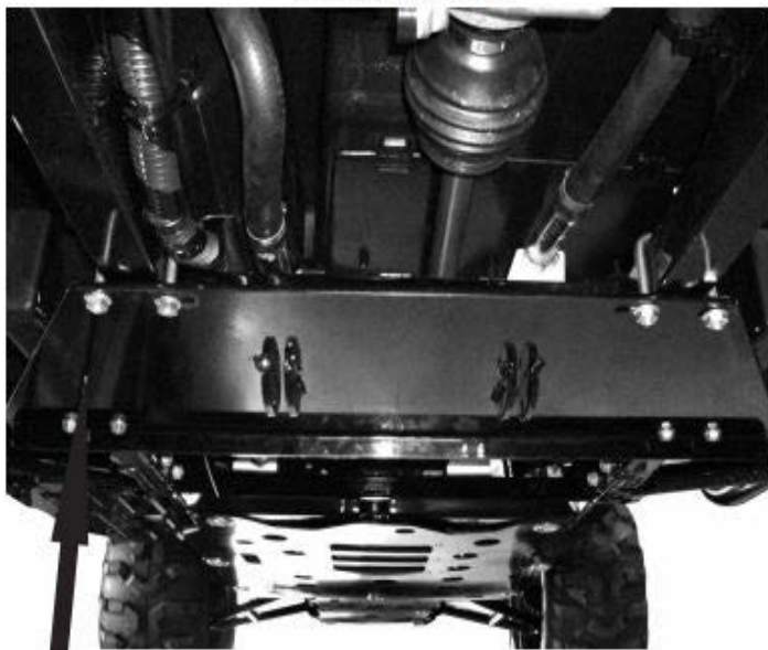
Front U-bolt position over the narrower part of the frame just in front of the horizontal frame member.
