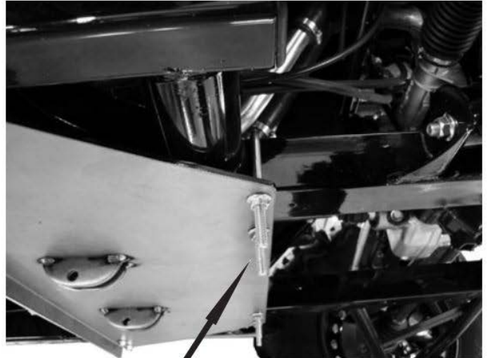
Front U-Bolt position over the square frame tubes where they are welded to the round frame crossmember.
