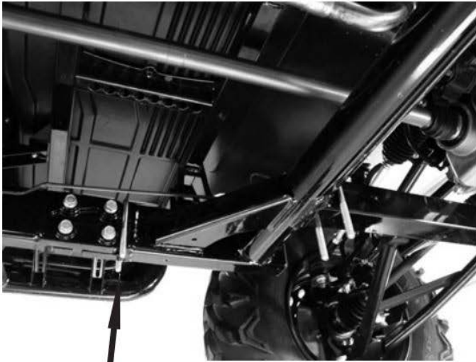
Rear U-Bolt position just in front of the four bolts holding the frame together
