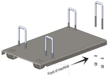
Push tube will pin up to plow mount tabs with wire loop pins that came with the push tube kit.
