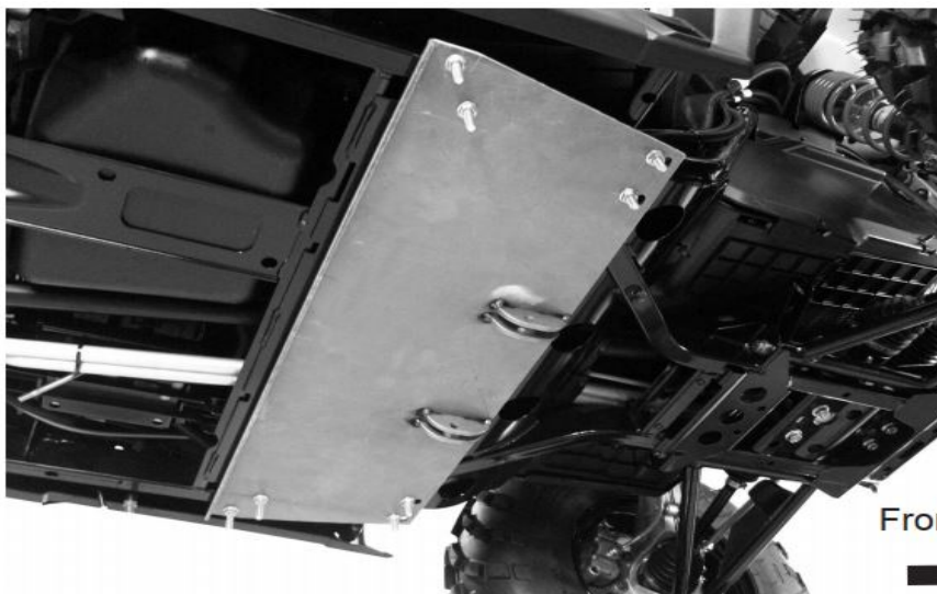
Rear U-Bolt position just in front of the horizontal crossmember.
