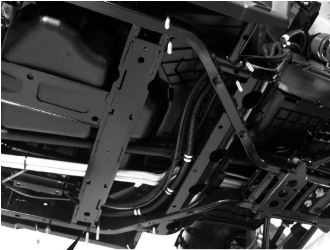
Rear U-Bolt position just in front of the horizontal crossmember.
