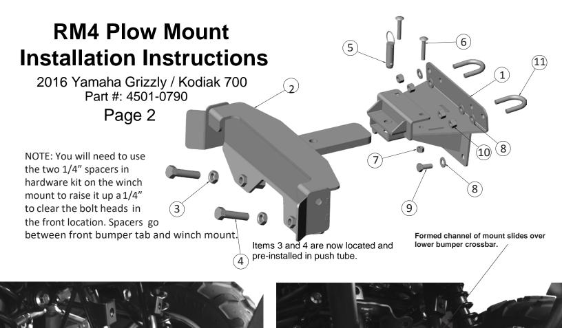
Bottom of mount bolts to the existing holes in the end of the frame tubes.
