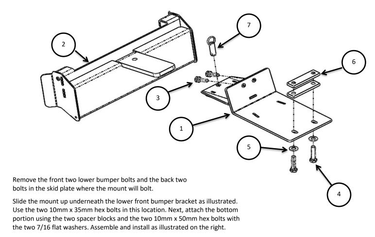
The removable mount will slide into main mount plate and secure with the cotterless hitch pin.
