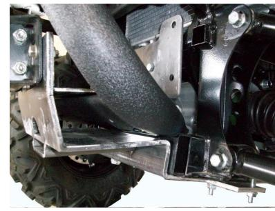
With the Yamaha winch mount you will need to use the RM4 mount as a guide and drill a 5/16 hole Through the Yamaha mount making sure your spacing is correct.
