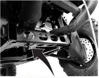
Install the included M10 bolts down through the bumper and frame.
