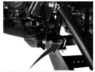
Place the u-bolts over the frame tubes just behind the front a-arm mounts.
