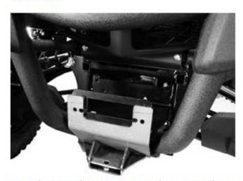
Line up the holes for the roller fairlead and install your fairlead through both plates.
