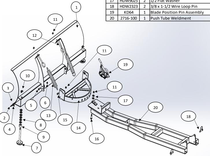
Install the blade swivel to the front of the push tubes using the ½"x 1" shoulder bolt, two ½" washers and one 3/8" nylock nut. Make sure swivel still turns after tightening (you may only need one washer).
