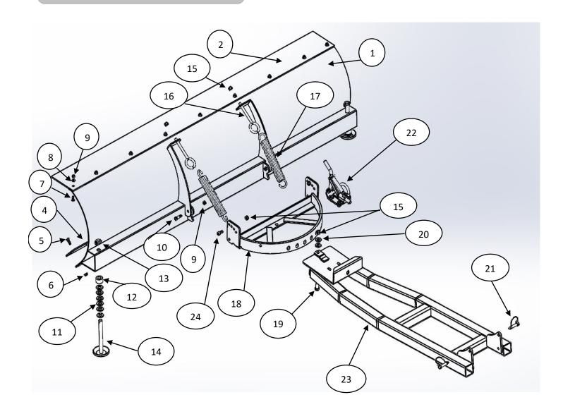
Install the blade swivel to the front of the push tubes using the  $\frac{1}{2}x 1^{"}$  shoulder bolt, two  $\frac{1}{2}$ " washers and one  $\frac{3}{8}$ " nylock nut. Make sure swivel still turns after tightening (you may only need one washer).
