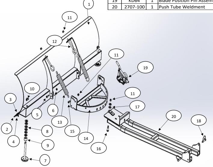
Install the blade swivel to the front of the push tubes using the  $\frac{1}{2}x 1^{"}$  shoulder bolt, two  $\frac{1}{2}$ " washers and one  $\frac{3}{8}$ " nylock nut. Make sure swivel still turns after tightening (you may only need one washer).
