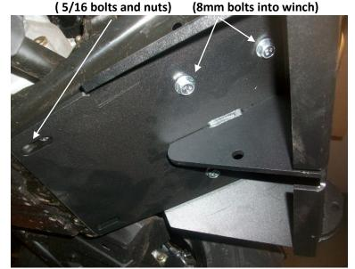
( Align mount up with winch mounting holes )
