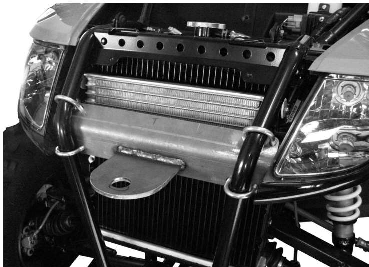
Bolt the winch hook bracket to the inside of the main frame tubes.
