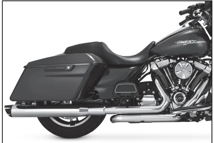
4. Align mufflers and tighten hardware, beginning with the 5/16" bolts on the mounting brackets as followed by the band clamp. Tighten 5/16" bolts to factory specs, and the band clamp to 40-45 ft./lbs.
