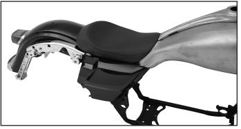
2. The stud and the jam nut should be loose in the bracket at this time. Adjust the grommet stud so there are approximately three threads out of the bottom; see REF. B. This will be a good starting point.
