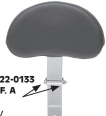
**WARNING:** Do not ride without the pad on the detent bar or the pad above the highest detent.
