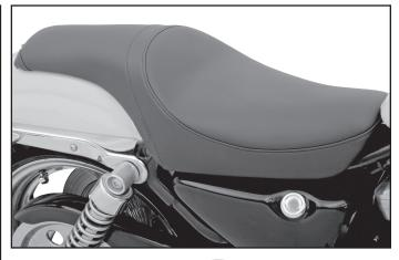
4. Slide your seat over the tab at the front of the frame near the gas tank, position the seat so it sits
