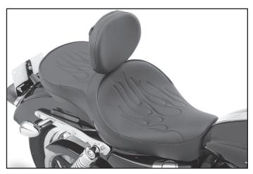
3. Loosen rear bracket slightly, install seat by inserting the front seat tab into the receiver behind the gas tank. Pushing seat forward, align rear bracket with hole in fender. Remove seat, tighten rear bracket and reinstall the seat using the Phillips-head screw previously removed.
