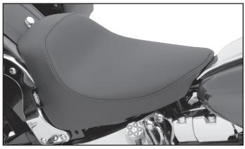
4. Slip your new seat over the tab at the front of the frame near the gas tank and position on the rear fender.
