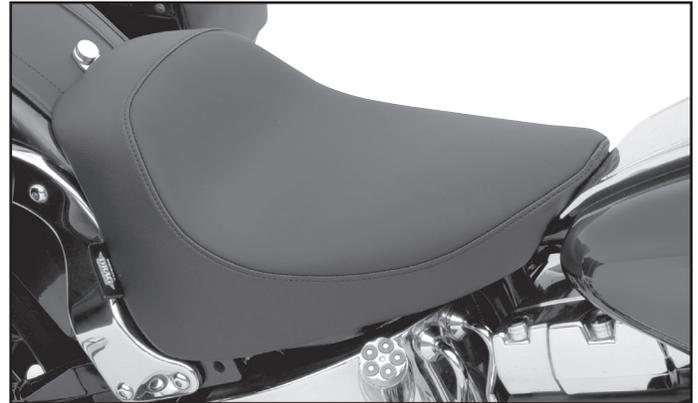
4. Slip your new seat over the tab at the front of the frame near the gas tank and position on the rear fender.
