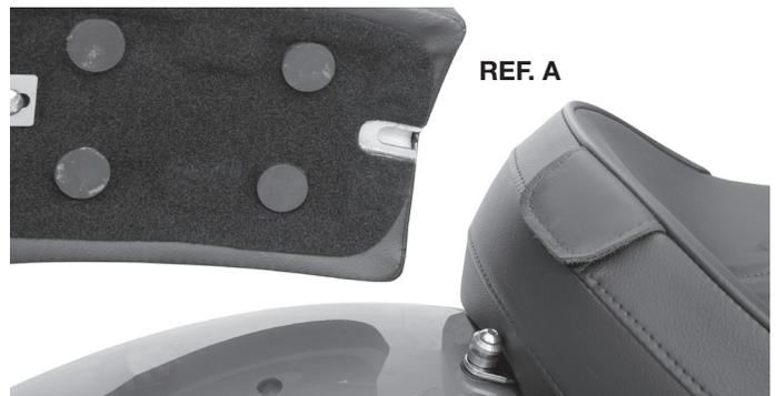
1. Remove the Solo front, rear mount screw. This screw will be reused on the Solo rear. Locate the Solo front receiver stud (**REF. A**) and reinstall over the bracket using the 1/4" x 20 x 1" button-head screw provided.
