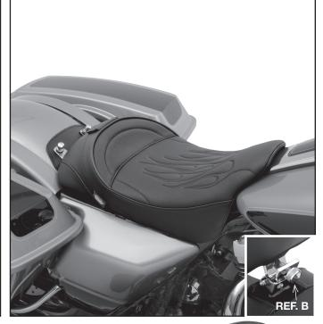
2. Position the front of solo over the two chrome dome nuts that secure the rear of the solo front.
