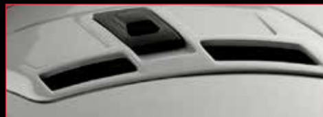
HIGH VOLUME INTAKE AND EXHAUST VENTS
