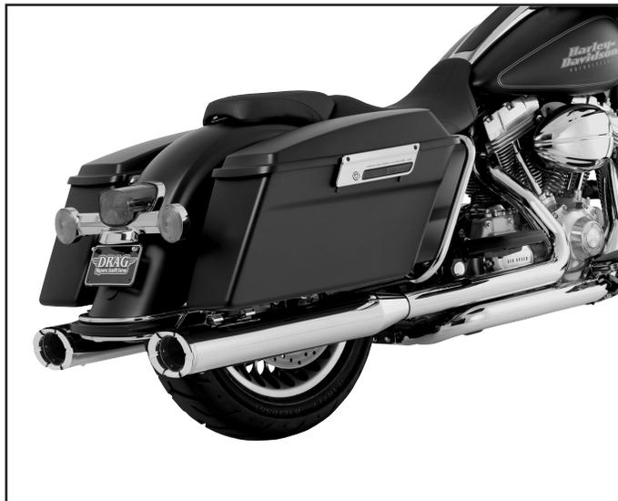
**NOTE:** There is a different muffler for the left and right side of the motorcycle. The dent in each canister should always be facing in towards the rear tire. This is to allow clearance for the swingarm and axle.
