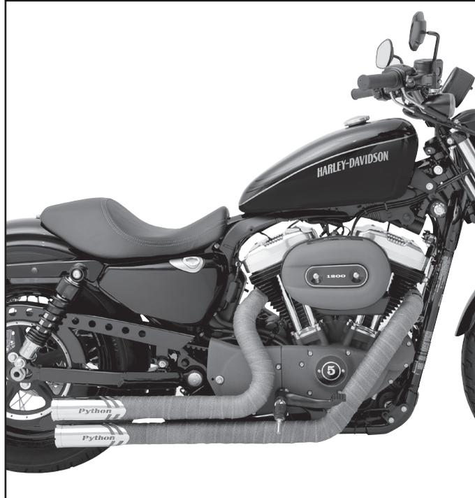
3. Remove the two headpipe mounting nuts from each flange, located at the cylinder head.
