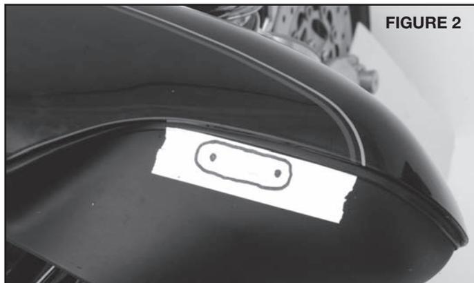
4. Position the mirror on the inner fairing so the scribed mounting hole marks line up with the mounting bracket. Have the rider confirm once again that the mirror is in the proper location.
