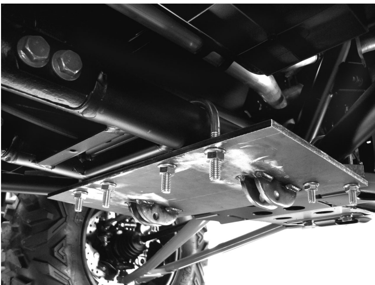
Place the bottom mount over the U-bolts and secure with the flat washers and nylock nuts.
