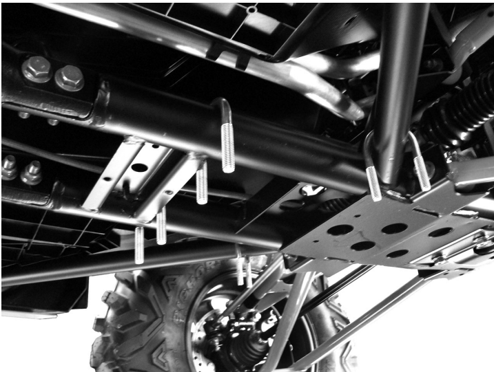
U-bolt placement on the frame tubes.
